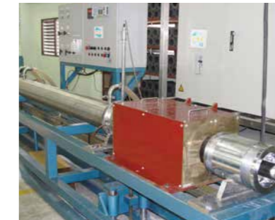
Bright Annealing Process After Form
